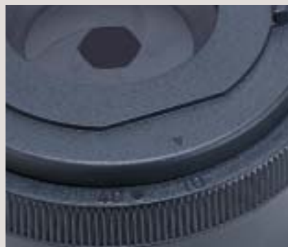
Field diaphragm with position-guide markings.
